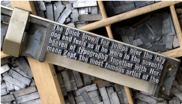
Four lines in a composing stick, set solid: no lead between them
